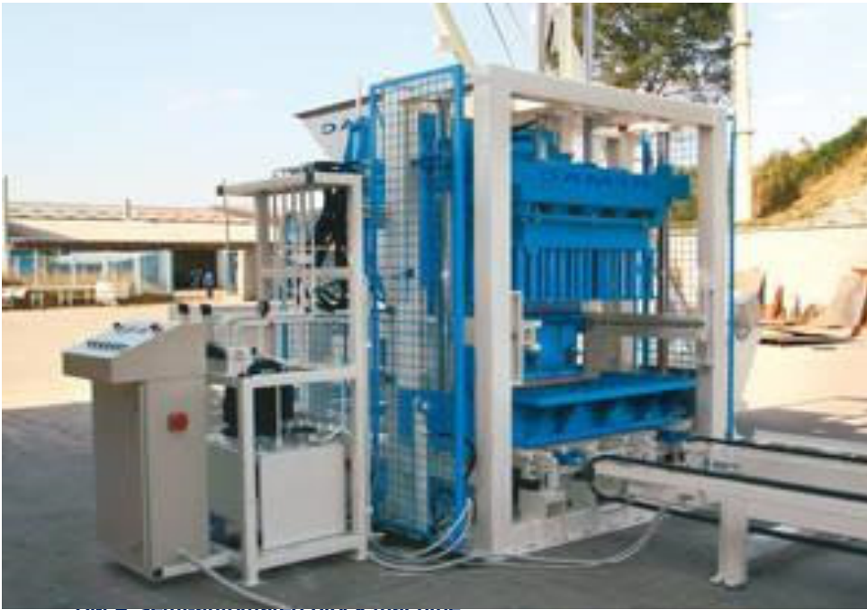
BM 4, Semi-automated block machine.
