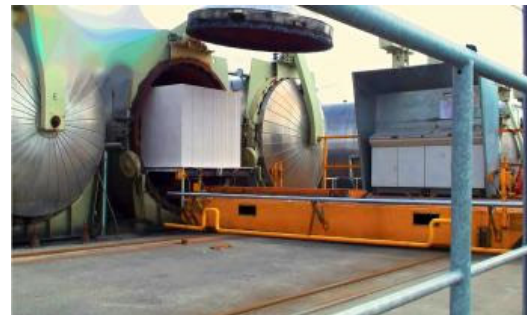
After 8 hours of curing time, the cured cake leaves the autoclave.
