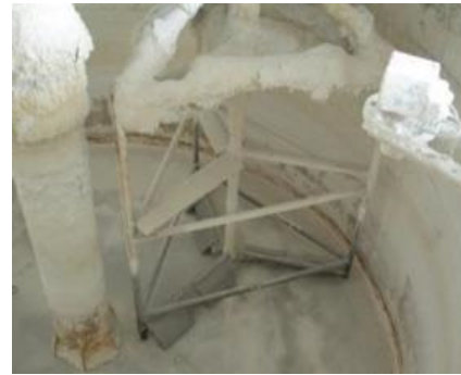
Silo of sand and quicklime of the water with agitator and measure of density.
