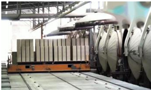
The importation of the green blocks in the autoclave
