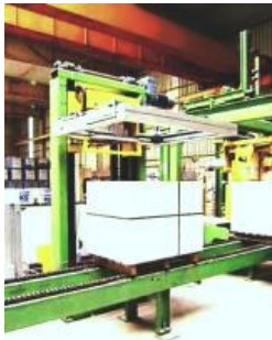
Strapping of sand-lime brick.
