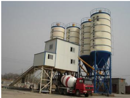
Concrete mixing plant single line
